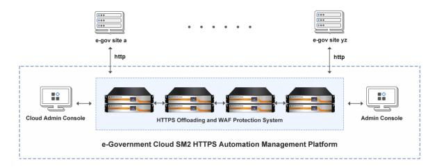
For the deployment of small and medium-sized websites, it is recommended to deploy at least two HTTPS Auto WAF Gateways to realize dual-machine hot backup and ensure uninterrupted 24 hours x 365 days of https encryption services. Two dual-system hot standby modes are optional:
